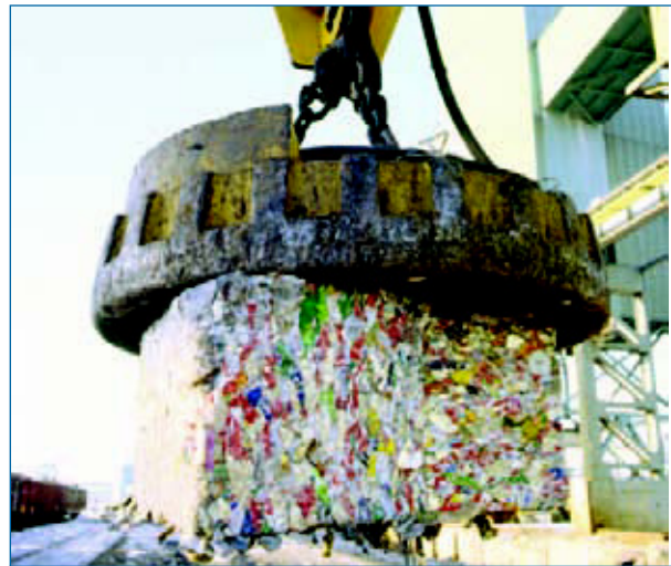
The magnetic properties of steel allow it to be easily separated from the waste stream.
